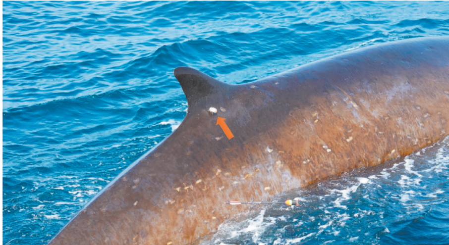
Figure 9. LIMPET-type SPLASH-F-333 (Wildlife Computers Inc.) was attached to the dorsal fin of a fin whale off the coast of Abashiri on 10 May 2022. The arrow-type carrier is also visible in the image.
