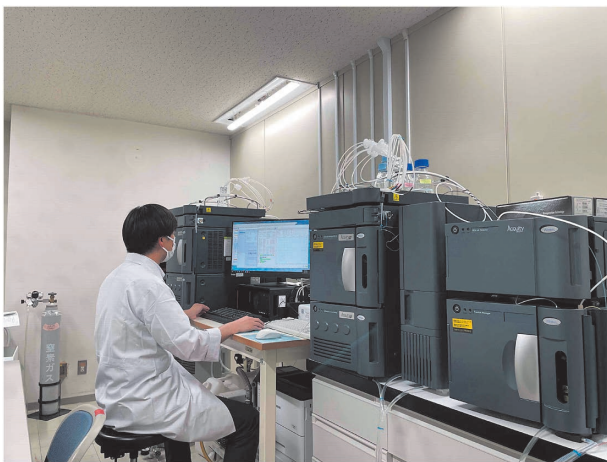
Figure 1. UPLC-MS/MS and FDA system at the environmental chemistry laboratory of the Institute of Cetacean Research.
