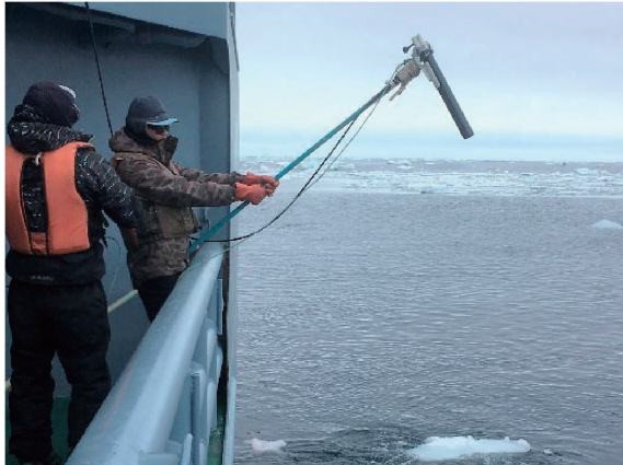
Figure 8. Oceanographic survey by XCTD.
