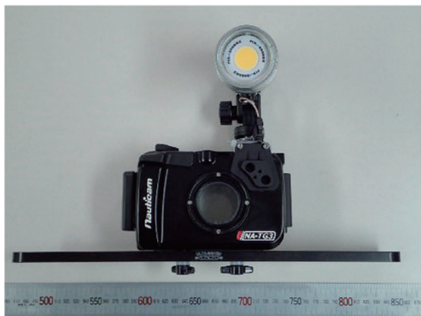
Figure 12. LED with camera used for attracting krill in the small sampling net.
