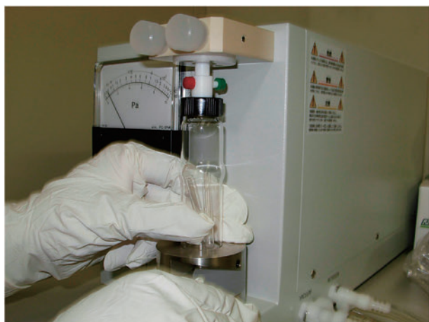
Figure 4. Hydrolysis of lens of Antarctic minke whale using Pico Tag Work Stations (Waters, Tokyo).
