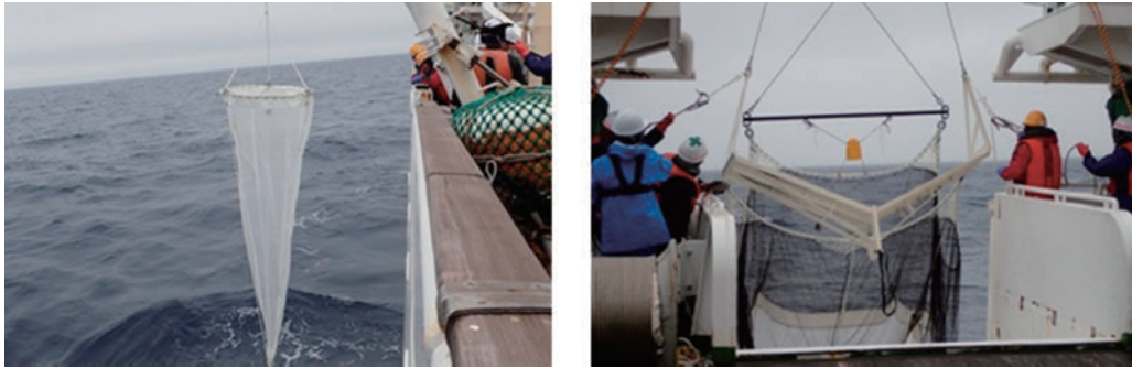
Figure 6. Small ring net (left) and an Isacs-Kidd Midwater Trawl (IKMT) net (right).
