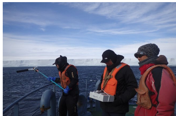
Oceanographic observation by XCTD near the ice shelf
