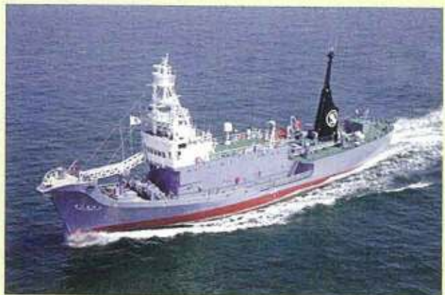
Fig. 15. The sampling/sighting vessel Yushin Maru No. 2. Joined the research fleet from 2002/03. Fitted with oceanographic research equipment, besides its capacity to perform sighting/sampling surveys (69.61m, 747 tons).
