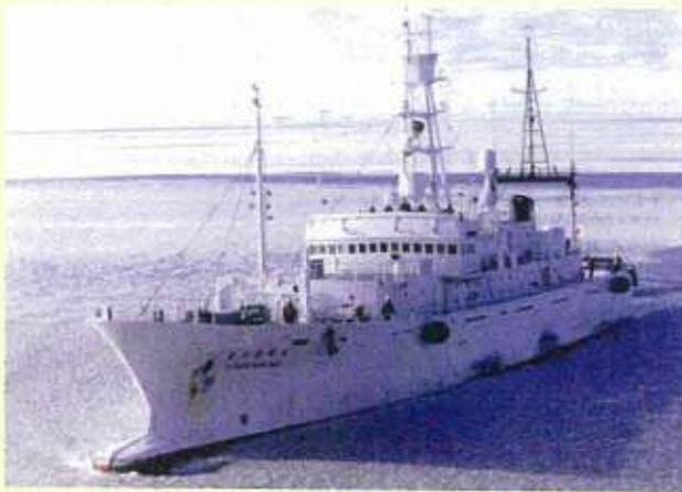
Fig. 12. The dedicated sighting vessel Kyoshin Maru No. 2 navigating ice floes in the Antarctic Ocean. Conducts echo-sound research on krill resources and oceanographic surveys besides sighting surveys (68.18 m, 372 tons).
