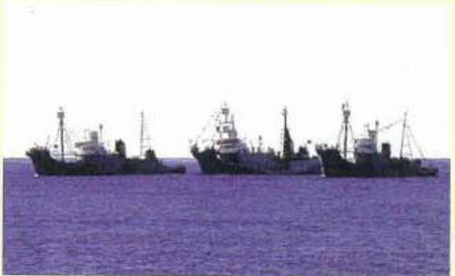
Fig. 17. Three sampling/sighting vessels sailing towards the research area in the Antarctic. Once the survey starts, a constant distance of 7 nautical miles is maintained between each of them.
