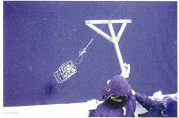
Fig. 76. CTD observations. The CTD is thrown into the sea to collect data on the vertical distribution of water temperature and salinity.
