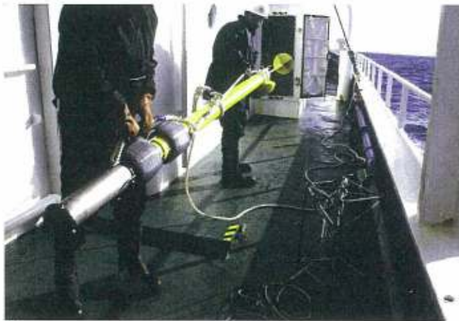
Fig. 82. Preparing the sono-buoy for deployment, aboard the sighting vessel Kyoshin Maru No. 2 .
