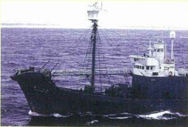
Fig. 14. The sampling/sighting vessel Kyo Maru No. 1. Since 1987/88 takes part every year in the JARPA program (69.15m, 812 tons).
