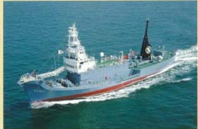
Fig. 16. The sampling/sighting vessel Yushin Maru No. 2. Joined the research fleet from 2002/03. Fitted with oceanographic research equipment, besides its capacity to perform sighting/sampling surveys (69.61m, 747 tons).
