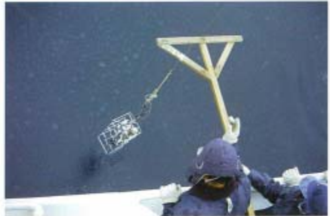
Fig. 76. CTD observations. The CTD is thrown into the sea to collect data on the vertical profile of water Conductivity (salinity), Temperature, and water pressure (Depth).
