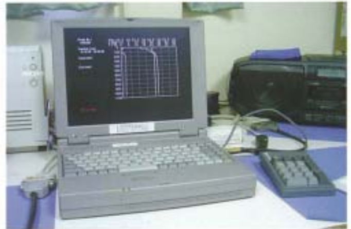
Fig. 22. XCTD data monitor. Oceanographic survey data are processed on board.
